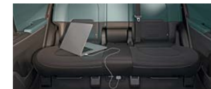
V2L - Vehicle-to-Load (Internal) (Only in X-Line)
